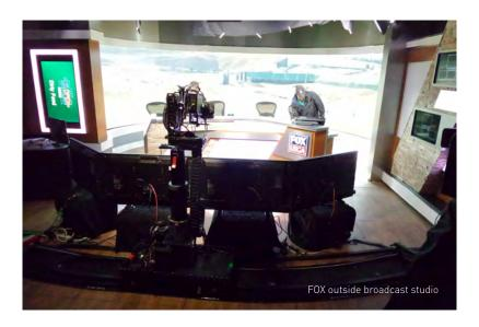
from the ground; the track itself is only 30 mm (1.18") from the ground, making it the lowest profile track design available on the market today. As a result, the network incorporated the Hexagon Tracks into their studio so that the space could remain "walkable" without anyone having to jump or trip on the equipment, while still providing the eye-level shots required.
