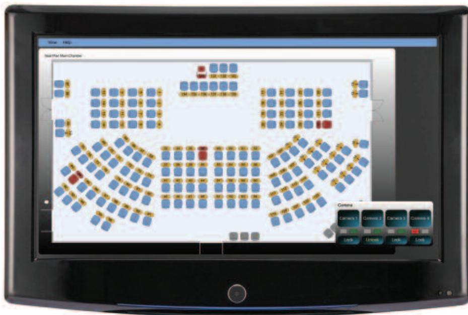
The Vinten Radamec **Legislative Control System (LCS)** provides multi-user, multi-facility control of cameras, CCU controls and robotics devices, ensuring rapid, accurate shot acquisition required to televise parliamentary and legislative procedures.
