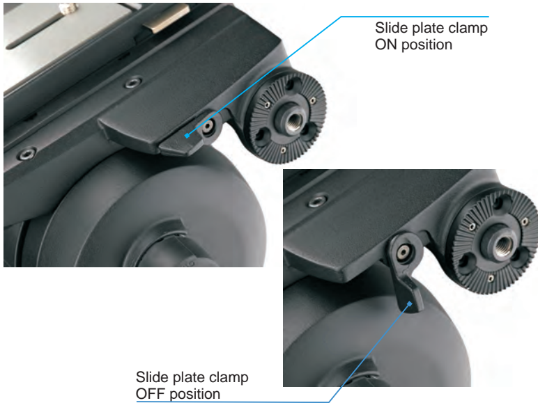
Fig. 8 Slide plate clamp (ON/OFF positions)
